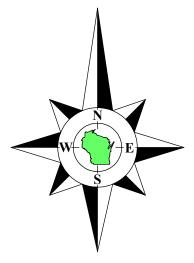
Bearings referenced to the North line of the Southwest 1/4 of Section 14-3-15, recorded as N87°11'15"E in the Wisconsin State Plane Coordinate System, South Zone, (NAD-27).
